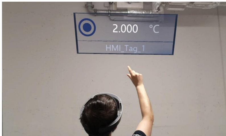
Figure 2-9: Real-time holographic dashboard showing the temperature of a pipe [17].
