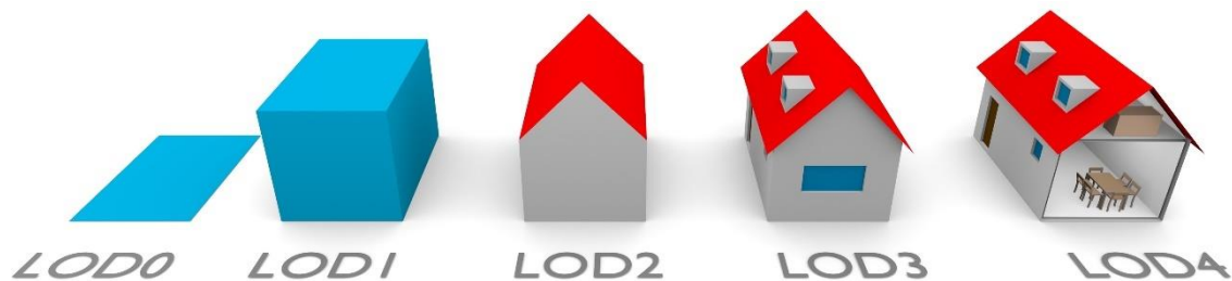
Figure 4-1: CityGML 2.0 building model classification based on LOD [48].
