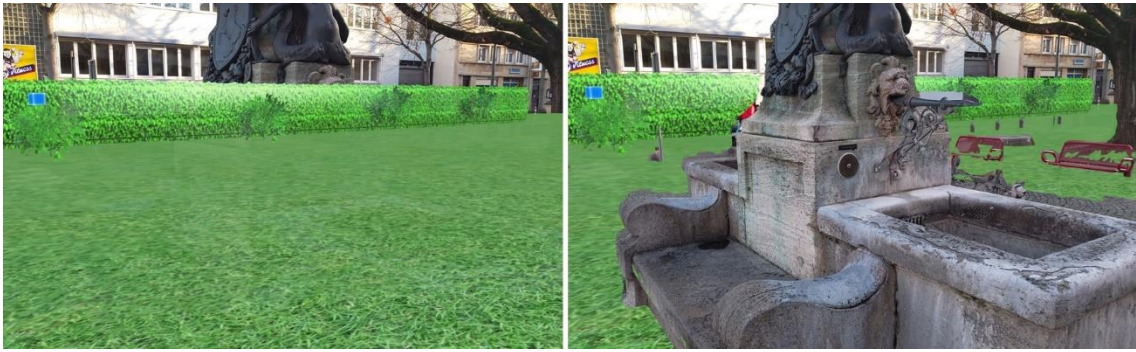
Figure 7-5: Occlusion screening based on the spatial map. ( left ) Disabled. ( right ) Enabled.
