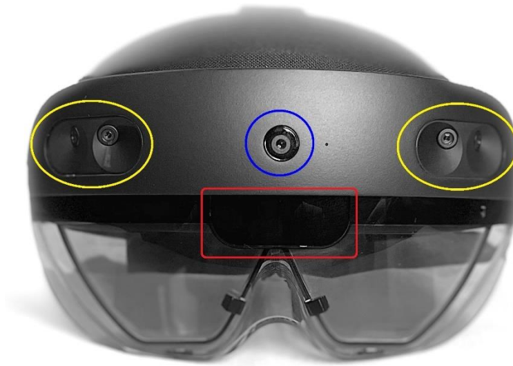
Figure 4-4: HoloLens 2.0 camera configuration. (yellow) Grayscale tracking cameras. (Red) ToF camera. (Blue) RGB camera.
