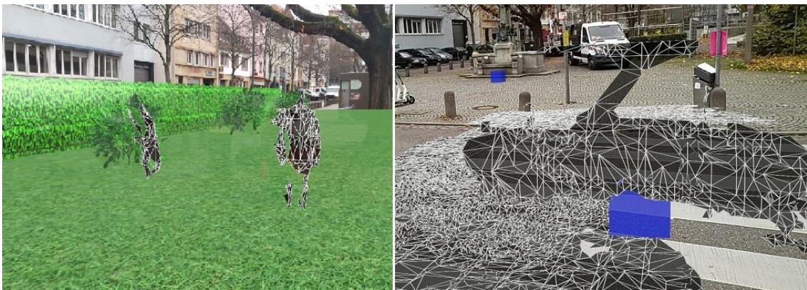
Figure 7-6: Noises during spatial map scanning caused by ( left ) moving pedestrians and ( right ) passing cars.
